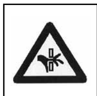
DANGER: RISK OF PINCHING OR TRAPPING !
