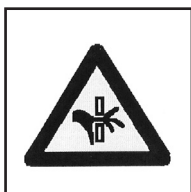
DANGER: RISK OF PINCHING OR TRAPPING !
